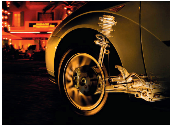
Figure 4.31 Suspension strut in position
